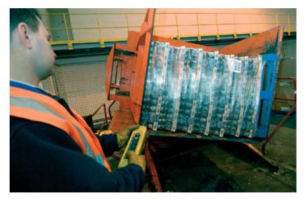
Figure 45 Pallet inverter
