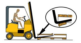
**(b)** Mast should not be tilted backwards until forks have fully entered and lifted the pallet
