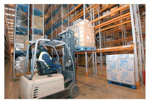
Figure 18 Counterbalanced fork-lift truck
