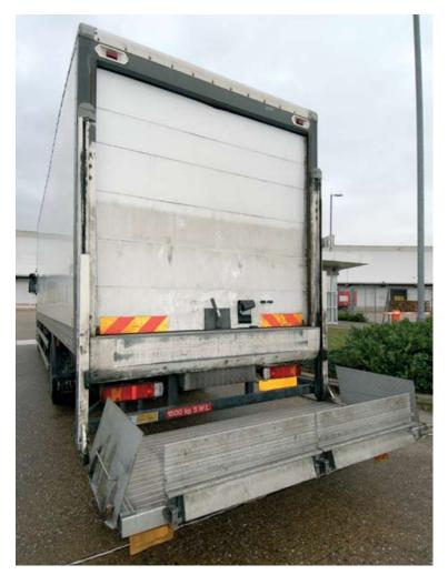
Figure 31 Vehicle with tail lift
