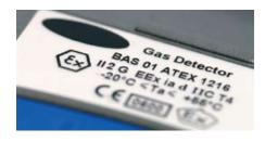
Figure 12 Ex marking showing that the equipment is explosion protected
