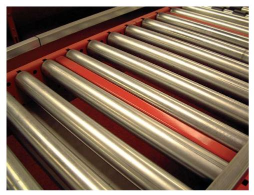
Figure 22 Roller conveyor
