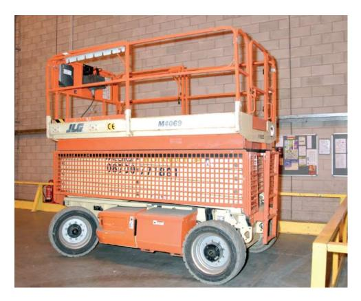
Figure 34 Mobile elevating working platform (MEWP)
