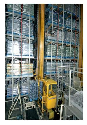
Figure 54 Rail-dependent storage and retrieval machine with operator cabin
