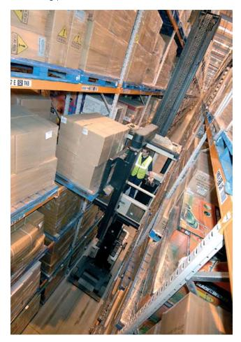
Figure 21 Very narrow aisle man-up truck
